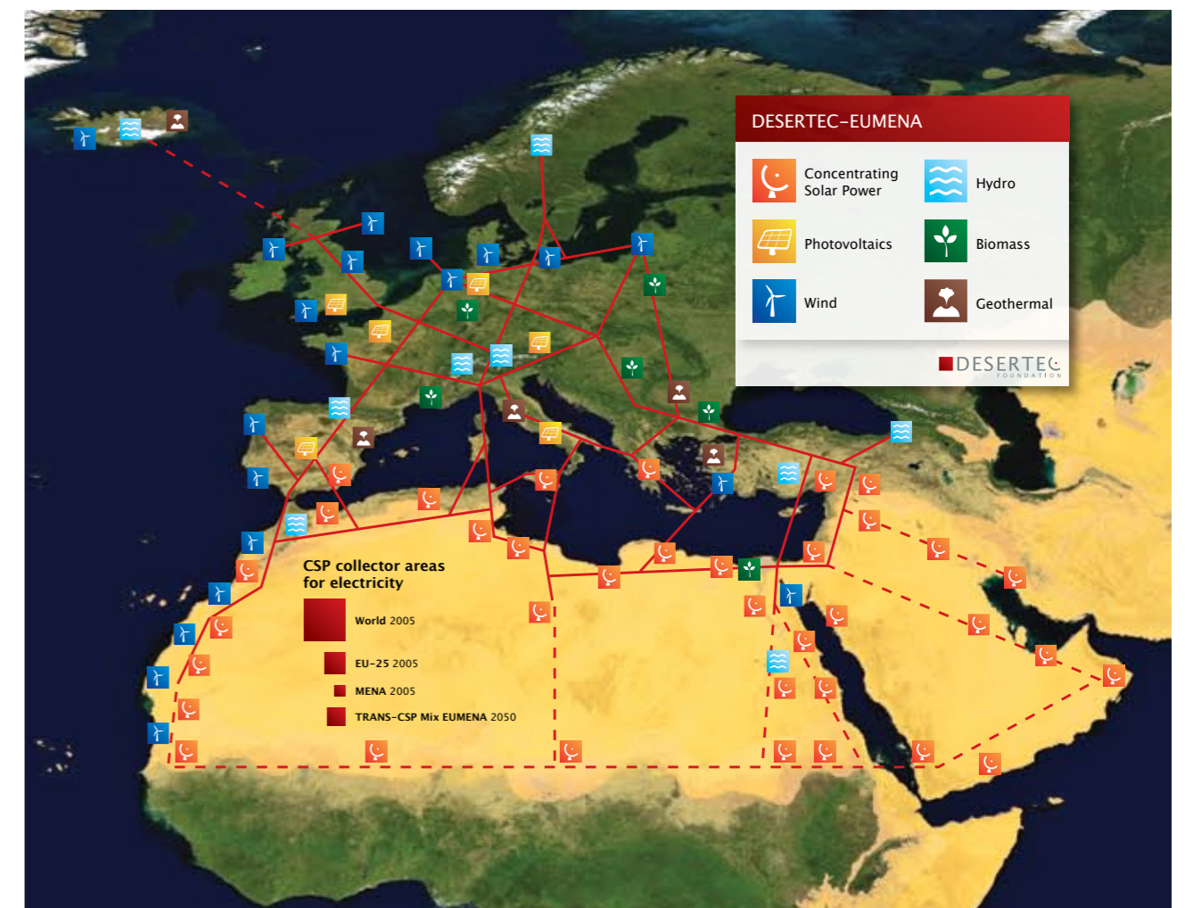
Figure 9: Concept of a "EUMENA Supergrid" based on HVDC power transmission as "Electricity Highways" to complement the conventional AC electricity grid, as developed by TREC in 2003. The symbols for power sources and lines are only sketching typical locations.
