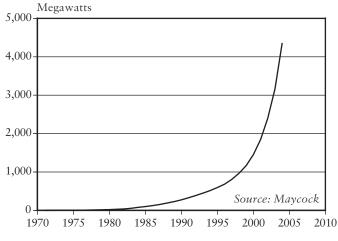
Figure 10–2. World Photovoltaic Generating Capacity, 1971–2004
